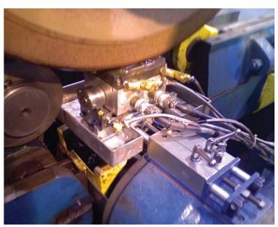
Inspection test head mounted on an underfloor profiling machine
