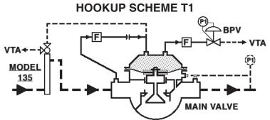
Use 1/4" tubing(ID of 0.180" or greater) when probe is installed within 18 feet of regulator.
