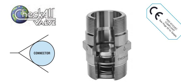
The **Connector (CN, CR)** value is a check value with a pipe nipple or connector housing. It is designed to be used in installations where a check valve with male pipe threads is required. The CN valve is adaptable for use as a low pressure relief valve or vacuum breaker by using the desired spring settings. Two valves used in combination make an excellent pressure vacuum vent. NPT threads are per ASME B1.20.1. Also available with ISO 7 "R" threads (CR).
