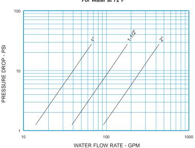
Horizontal-Vertical Flanged & Drilled PTFE Lined For Water at 72°F
