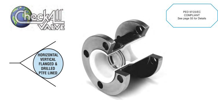
The **Check-All**<sup>®</sup> **Flanged & Drilled — Fluoropolymer (PTFE) Lined (HT)** check valve is a one piece body with ANSI/ASME B16.5 Class 150 flanged ends. The valve has a solid one piece PTFE liner which covers the flange faces out to the raised face diameter. All wetted surfaces are fluoropolymer (PTFE/FEP/PFA) including the FEP encapsulated stainless steel spring.
