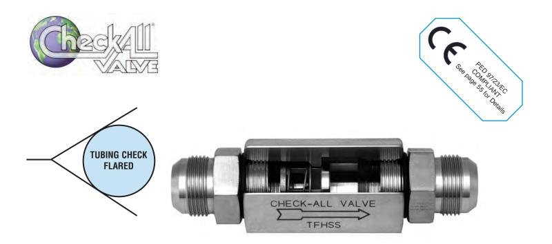
The **Tubing Check Valve-Flared (TF)** is a three-piece constructed check valve with 37° flared end fittings that conform to SAE J514 & ISO 8434-2. These valves are designed for maximum flow with minimal pressure drop. The TF valve can also be used as a low pressure relief valve or vacuum breaker by using the desired spring settings.
