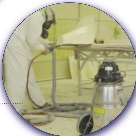
*The collection of hazardous debris in a manufacturing plant.*
