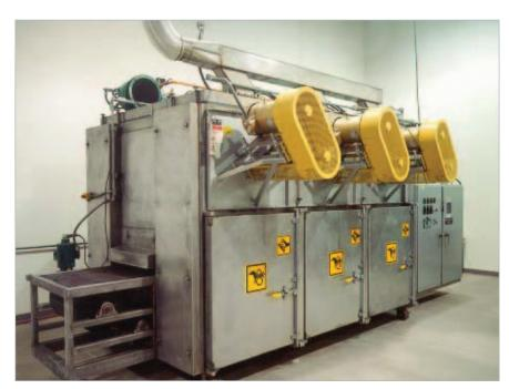
Portable pilot plant design is available with a variety of heating, conveying and air delivery configurations.
