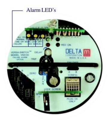
In normal operation, the channel two relay contacts are open and three yellow LED's are illuminated indicating an "Alarm Ready" status. If a failure occurs, the failure alarm relay contacts will close and one or more of the yellow LED's will be extinguished. The combination of "Off" and "illuminated" LED's will provide an indication of the probable malfunction. The column on the right side of this page indicates the possible light combinations and the potential malfunctions that they represent.
