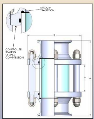
hese sterile design visual flow indicators provide operators with a full 360° view of nearly any process pipeline fluid flow while imposing virtually no pressure drop in the line. Electropolished stainless steel heads with a standard SF4 finish are available in sanitary clamp, orbital weld, Swagelok TS, flange, union or special order connection styles.
