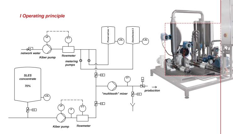
The diagram explains the production process:
