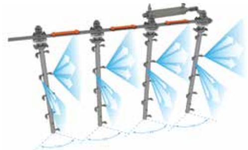
Spray bars oscillate 120° to provide complete cleaning coverage
