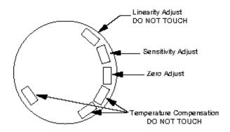
Linearity - DO NOTTOUCH - Factory adjusted for best linearity. Touching any adjustments other than zero output or sensitivity may necessitate recalibration.
