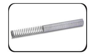
Open/closed coil hose guards are designed to act as a bend restrictor behind the coupling attached on the hose. This protects the hose from being bent too excessively behind the coupling. Each coil has a closed end which enables firm attachment onto the coupling. Each coil is constructed of steel wire and plated with a zinc coating to resist rust. Warning tags available also.
