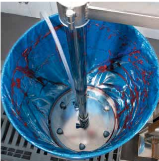
VISCOFLUX mobile – ideal for transfer out of conical drums with aseptic bags (example: Pharma Food Cosmetic version).
