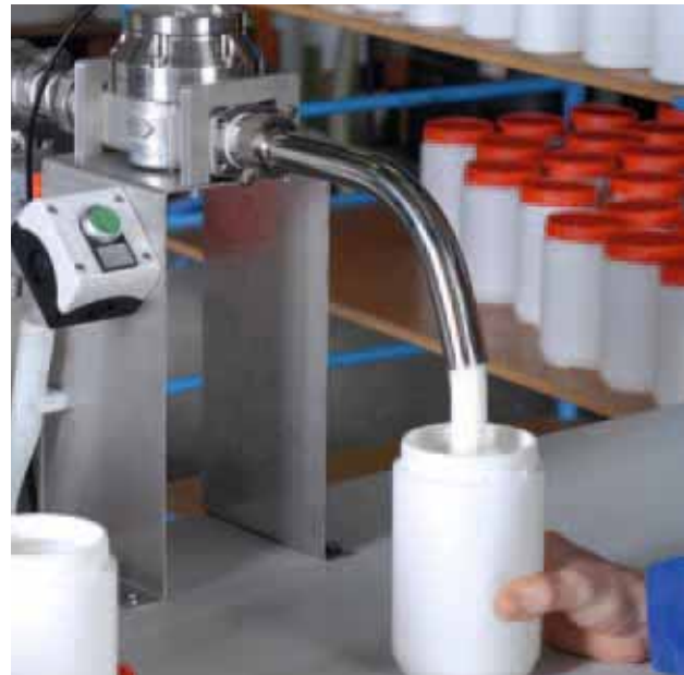
VISCOFLUX mobile – continuous transport (example: Vaseline).
