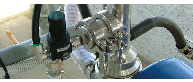
The Milk Recovery System ensures most of the residual milk in your system is emptied into the bulk tank at the end of milking.
