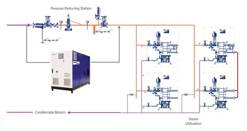
The compact design makes the Spirax TurboPower suitable for retrofitting into many existing steam plants – they are supplied fully assembled and tested to minimise on-site disruption.
