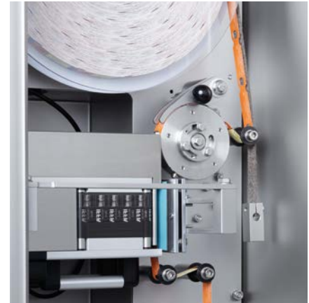
Compensating roller system ensuring the accurate position of the imprint
