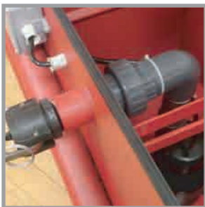
Return pump allows liquid return at 38 gallons/minute.
