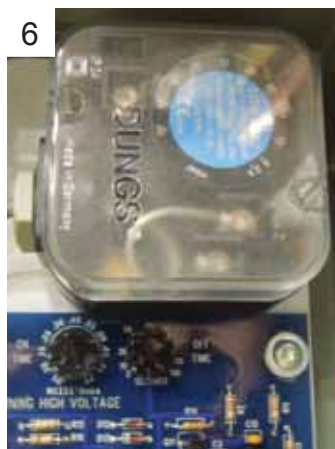
6 Replace the pressure switch snap-on cover.
