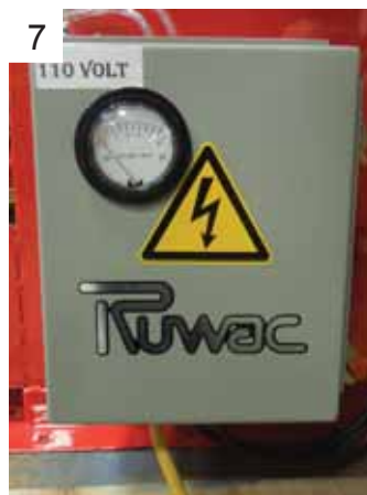
7 Close the reverse-pulse control box.
