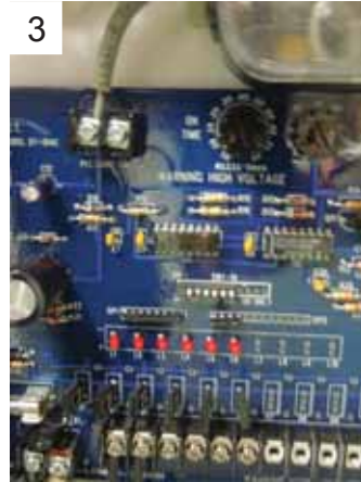
3 Set the left dial on the reverse pulse circuit card to 8 seconds. Set the right dial on the reverse pulse circuit to 0.1.
