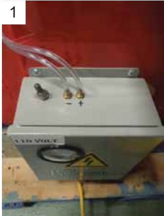
1 Turn the vacuum system off and disconnect the power source.
