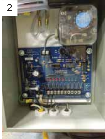
2 Open the reverse-pulse control box.
