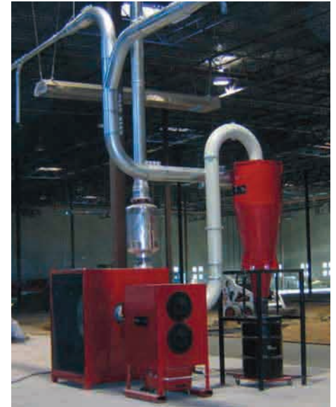
Above: FA2000 Filtration System as part of a central vacuum system, complete with a High Efficiency Cyclone pre-separation system.
