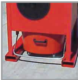
Forklift pockets allow filtration system to be easily moved into desired location.
