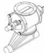
Convey Transition Feeds material into airstream to assist conveying.
