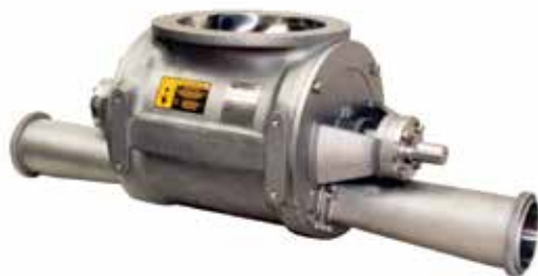
a) Blow through (CV) Product discharges horizontally at 90° to inlet via a pneumatic conveying line, either vacuum or pressure.
