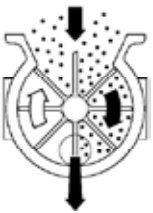
a) Blow through (CV) Product discharges horizontally at 90° to inlet via a pneumatic conveying line, either vacuum or pressure.
