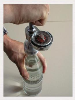
In the food & beverage industry, the opening torque of bottles and other containers with twist-off closures is an important quality parameter and vital for customer satisfaction.
