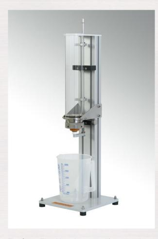
The Spout Flow Meter is a means for comparing (and measuring) the flow resistance of so-called "sport closures".
