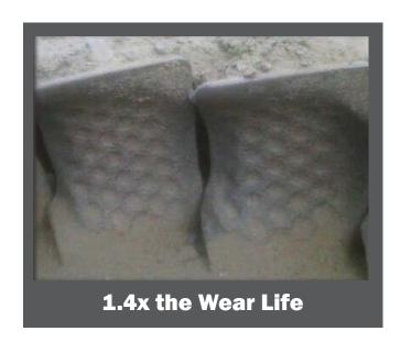
**Application:** Vertical shaft impactor - 24 piece anvil ring
