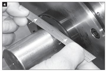
Make sure stator and rotor are flush.
