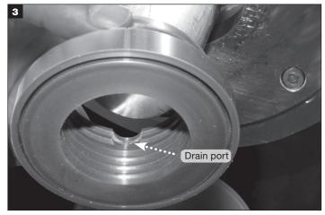
Apply a thin film of lubricant to the shaft and bore. Align the drain port at 6 o'clock position and slide the seal onto the shaft uniformly pressing both stator and rotor in the equipment.
