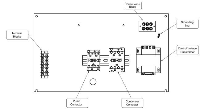
**Figure 14: Typical SMC Subpanel**
