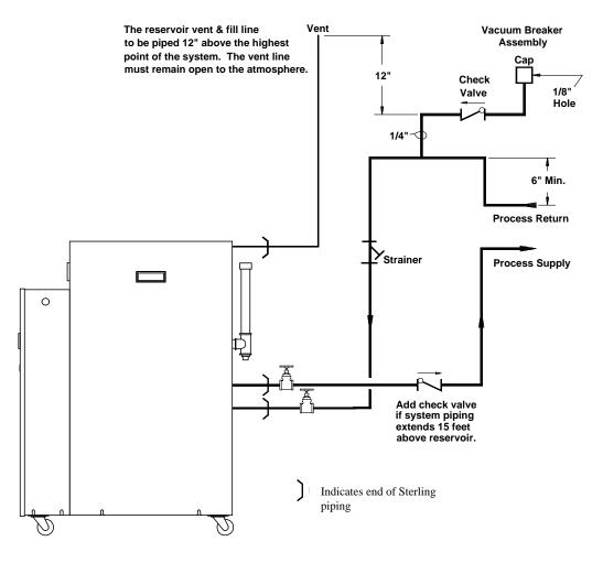
Figure 7: Overhead Piping
