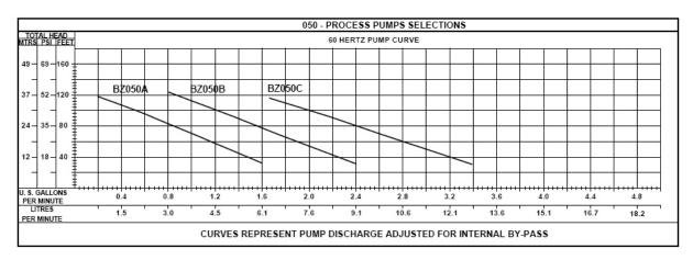
Figure 2: SMC100 Process Pump Curves
