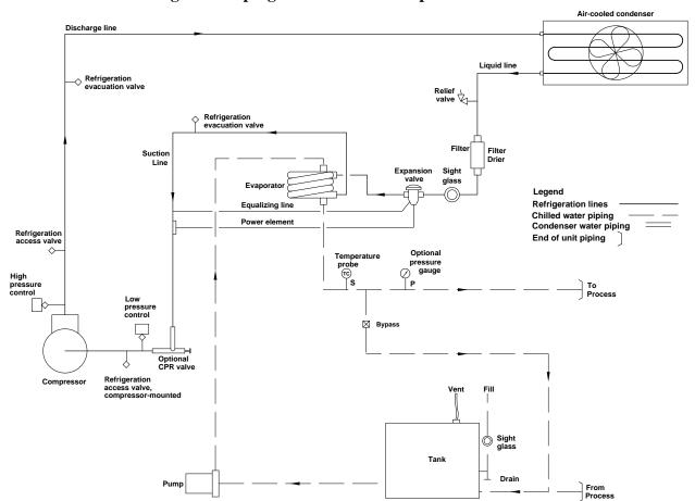
Figure 9: Piping Schematic - 1 Pump with Reservoir
