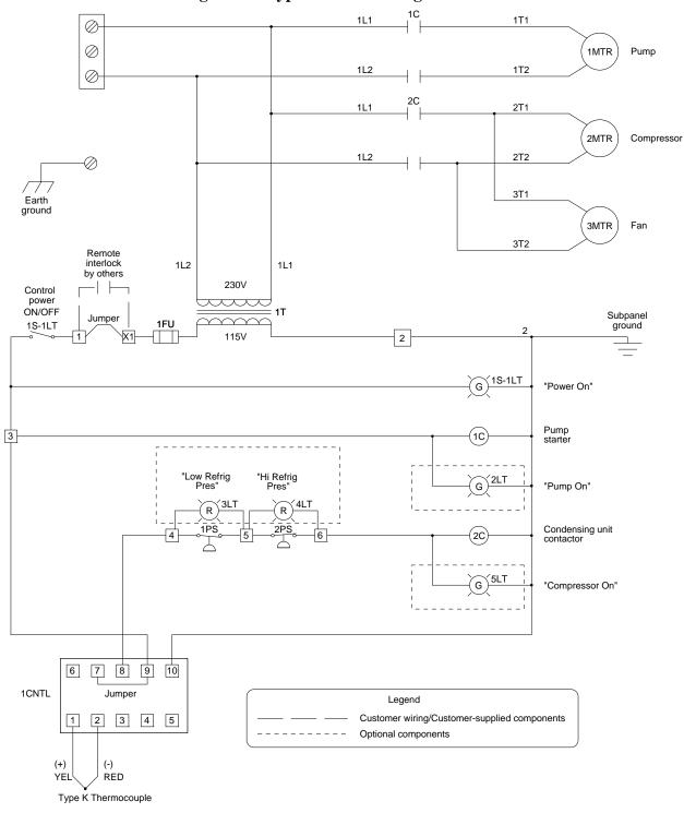
**Figure 15: Typical SMC Wiring Schematic**
