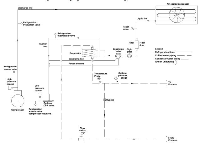
Figure 11: Piping Schematic - No Pump, No Reservoir
