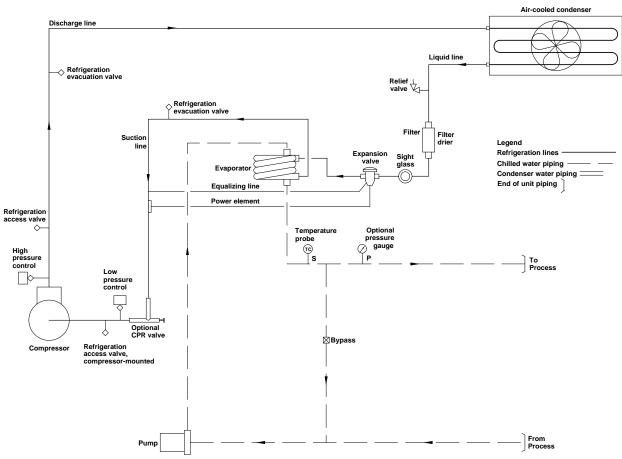
Figure 10: Piping Schematic - 1 Pump Without Reservoir
