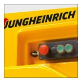
Inching buttons for simple coupling and decoupling
