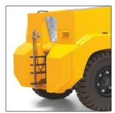
Multi-stage coupling for different trailer coupling
