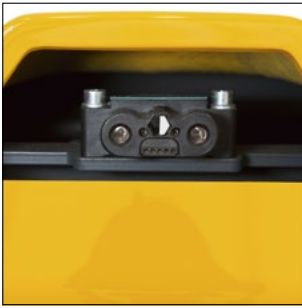
Electrical connection for trailers.
