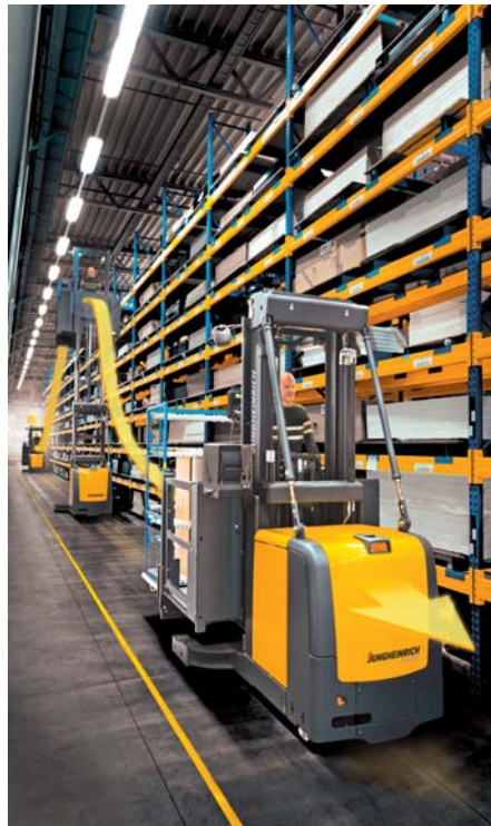
Synchronized material and information flow in the narrow aisle: Semi-automatic approach to order-picking positions with an EKS vertical order picker and warehouse navigation
