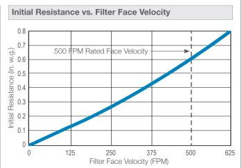
Recommended final resistance for all BioCel® VXL filters is 1.5 in. w.g.
