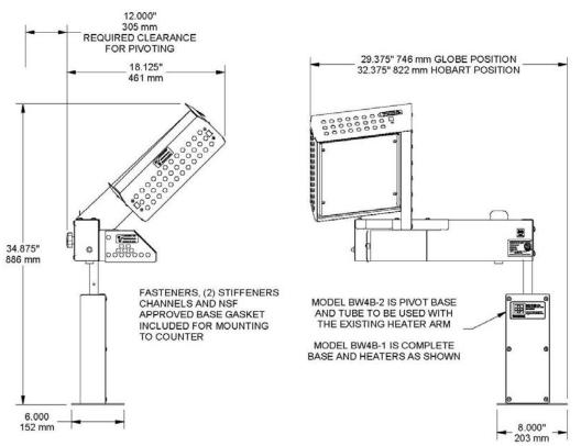
BW4B-1 is shown without slicer BW4B-2 consists of the pivot base only
