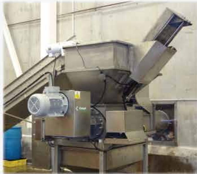
Waste Control International Screw Compactor can either be hand loaded or conveyor fed.
