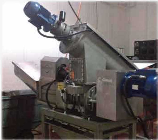
Waste Control International Screw Compactor can either be hand loaded or conveyor fed.
