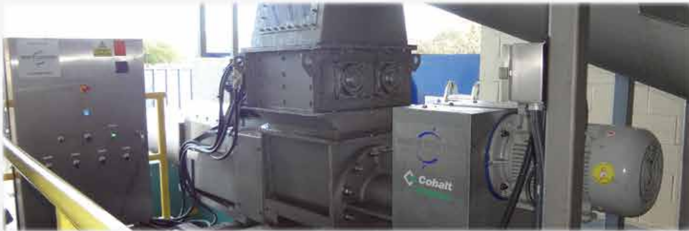
With a high volume of PET an optional perforator will puncture all the bottles before they enter the compactor chamber.
