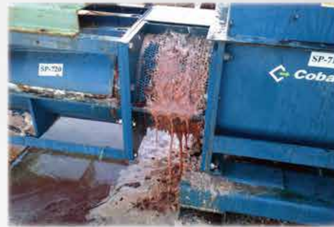
The screen area allows for maximum liquid flow. This helps achieve 99% liquid removal in a liquid destruction application.
