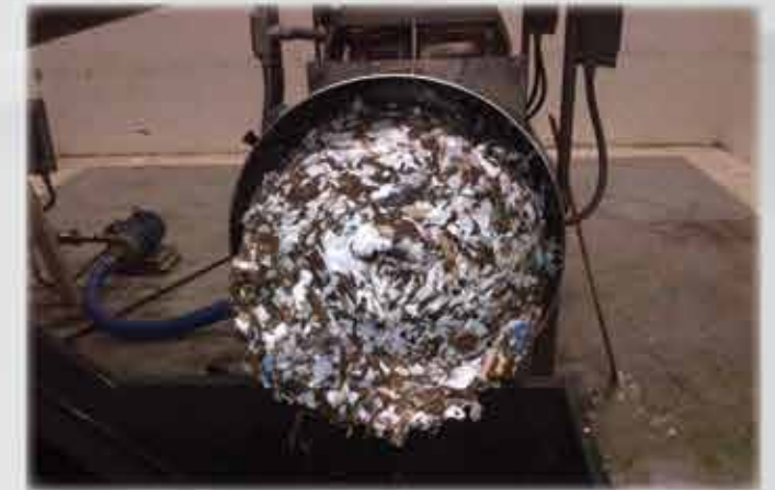
With compacted PET this screw compactor will put 600-800 lbs. of plastic into a box. This Screw Compactor will also allow you to get full weight on trucks going to the WTE Facility.
