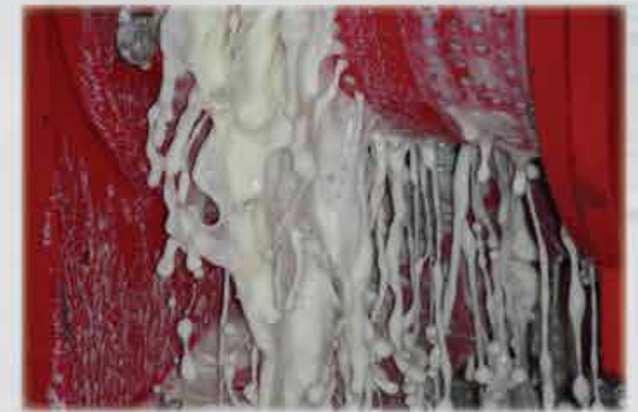
The screen area allows for maximum liquid flow. This helps achieve 99% liquid removal in a liquid destruction application.
